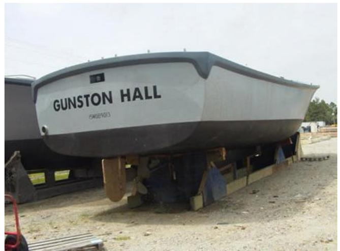
50 ft Willard Marine Utility Boat. Fiberglass construction. L: 50 ft; H: 12 ft; Beam: 14 ft. Weight: 24,000 pounds including crew and fuel. 146 person capacity.
